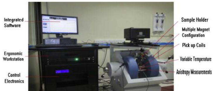
FIGURE 4 OPERATING PRINCIPLE OF VSM [7]
